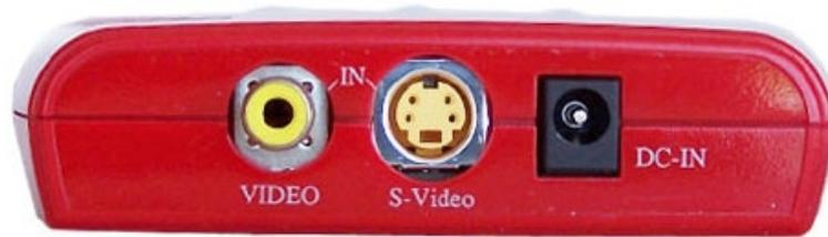
1. **DC-In-** This is the power supply input port. Connect it to the power adapter.
