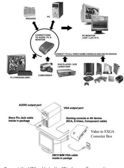
1 . Connect the VGA cable to the [Display card] connecting port on the PC system and the Video to SXGA Converter Box [VGA-IN I To PC]
