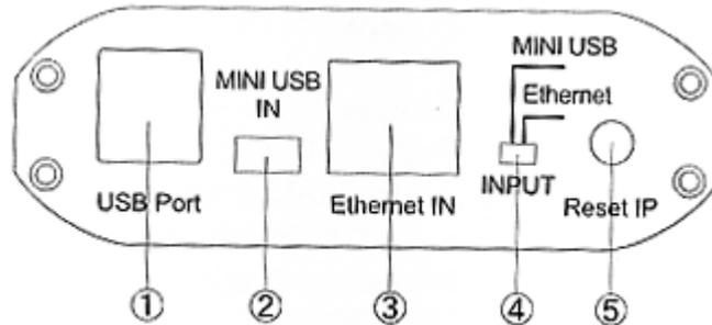
**1. USB Port:** Connect USB device into USB port such as, USB Hard Drive, USB web camera, Keyboard or Mouse.
