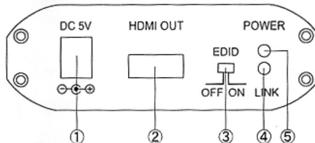
**1. Power:** Plug the 5V DC power supply into the unit and connect the adaptor to AC wall outlet.
