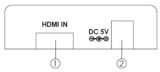
(1) **HDMI In:** This slot is where you plug in your source equipment such as settop-box or DVD player with HDMI cable.
