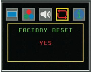
Select YES to return to the factory setting. Factory setting on display is at 1024 x 768@60Hz with full size screen, Color setting's factory default rate are as the value in the bracket of the OSD chart and SDI audio is on auto.
