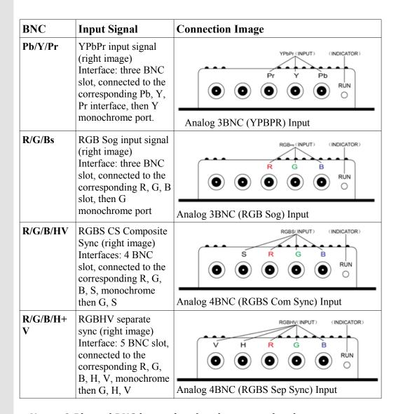
Note: 9 Pin and BNC input signal, only one can be chosen
