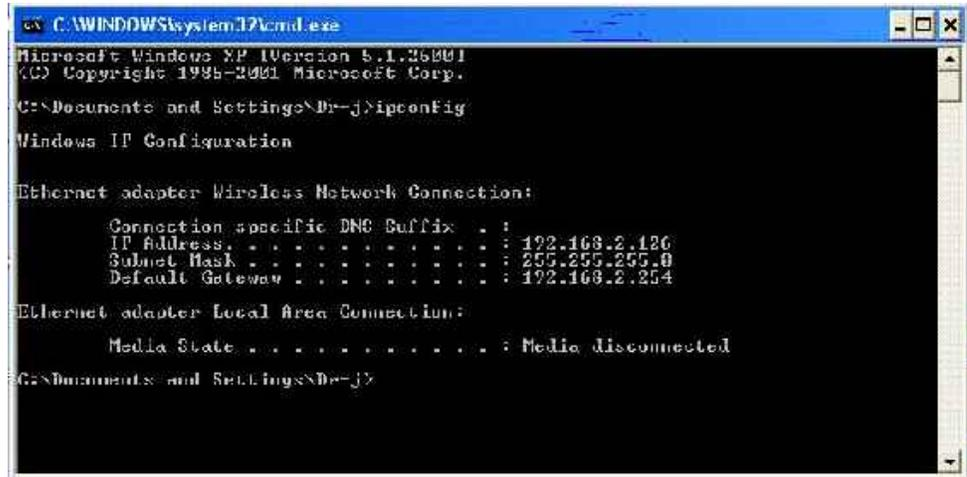
**Step 4 :** Then you can assign IP Address, Netmask (Subnet Mask) and Gateway (Default Gateway) for the IP Controller.
