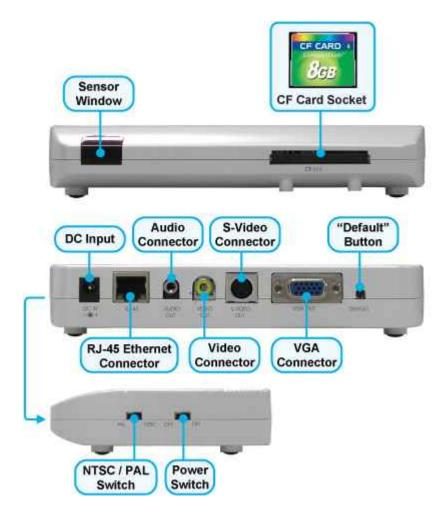
**IR SENSOR**: Infrared input of remote controller.
