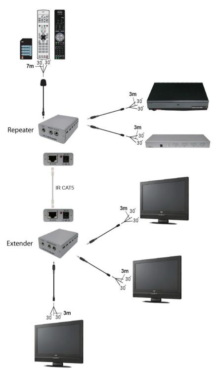
**Note: A.** IR receiver's control distance can goes up to 7 meters long with open space and direct angle.
