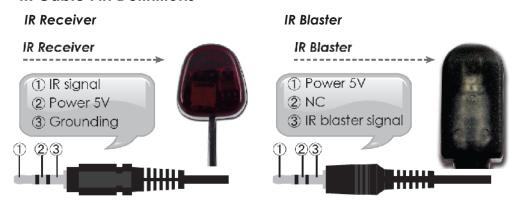
Note: Both the IR Receiver & Blaster can support a frequency of 20~70KHz.
