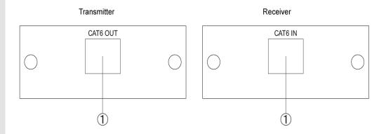
① CAT6 OUT/IN: Connect the CAT6 output of the transmitter with a CAT6 cable to the CAT6 input of the receiver.
