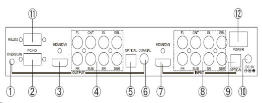
① **OVERSCAN:** When output timing is 480i59/60,480p59/60, 576i50 or 576p50, the output signal may not showing full image on the screen, press the OVERSCAN button to fill screen completely.
