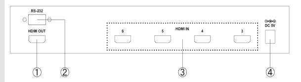
(1) HDMI OUT: This is the slot where you connect the HDMI output of the switcher to the HDMI input of your display using a HDMI cable.
