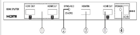
**1. HDMI OUT 7/8/1:** Using HDMI cables connect these slots to displays in order to show HDMI/3D content.
