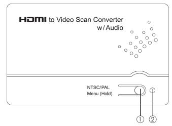
1. NTSC/PAL MENU (3SEC): Press this button to bring up the OSD which will display the input timing and output TV system information.
