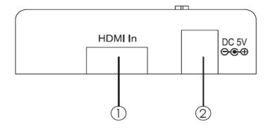
**1. HDMI IN:** This slot is to connect to the HDMI source equipment such as PC/NB with HDMI output and the connection cable for input signal sending.
