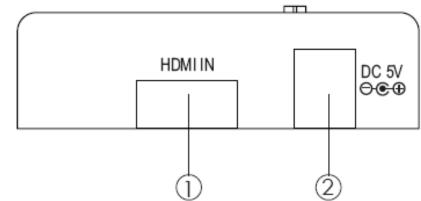
**1. HDMI IN:** This slot is to connect with input source equipment such as DVD or Blue-Ray player with HDMI cable.
