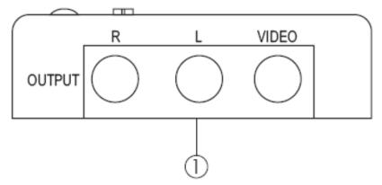
**1. OUTPUT R/L/VIDEO:** These slots are to connect with output display TV/monitor with R/L & composite RCA jack cable.
