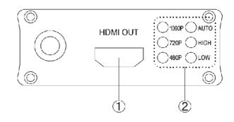
(1) HDMI out: Scaled digital HDMI output. Connect this output to the HDMI display and the output resolution support -1080p, 720p and 480p.
