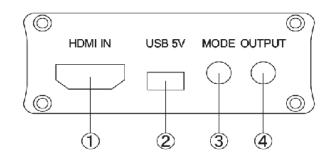
(1) HDMI IN: Connect this HDMI input connector to the HDMI output connector of your HDMI source equipment using certified HDMI cable or connect this HDMI input connector to the DVI output of your DVI source equipment using DVI cable together with DVI to HDMI adaptor. The HDMI input resolution support 480i~1080p and VGA~WUXGA.
