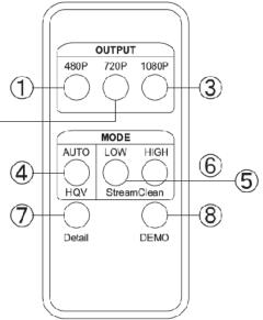
⑦ Detail: Toggles between Resolution Enhancement On and OFF.
