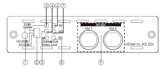
① **EDID Update button:** Use this function only when the image does not display after trying to switch the EDID/HD/3G EDID swtich.
