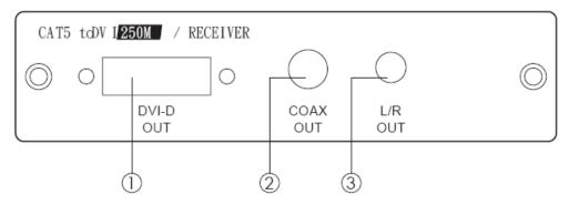
① **DVI-D OUT –** Connect to DVI/HDMI display equipment with DIV or DVI to
