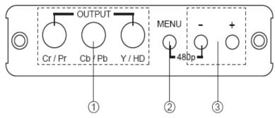
**1 Component output:** Connect the component output port to the component input port of your display.
