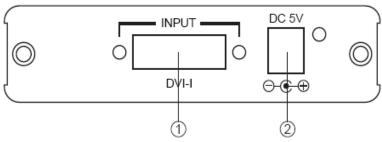
**1 DVI-input:** Connect the DVI-I input port to the output port of your source equipment.
