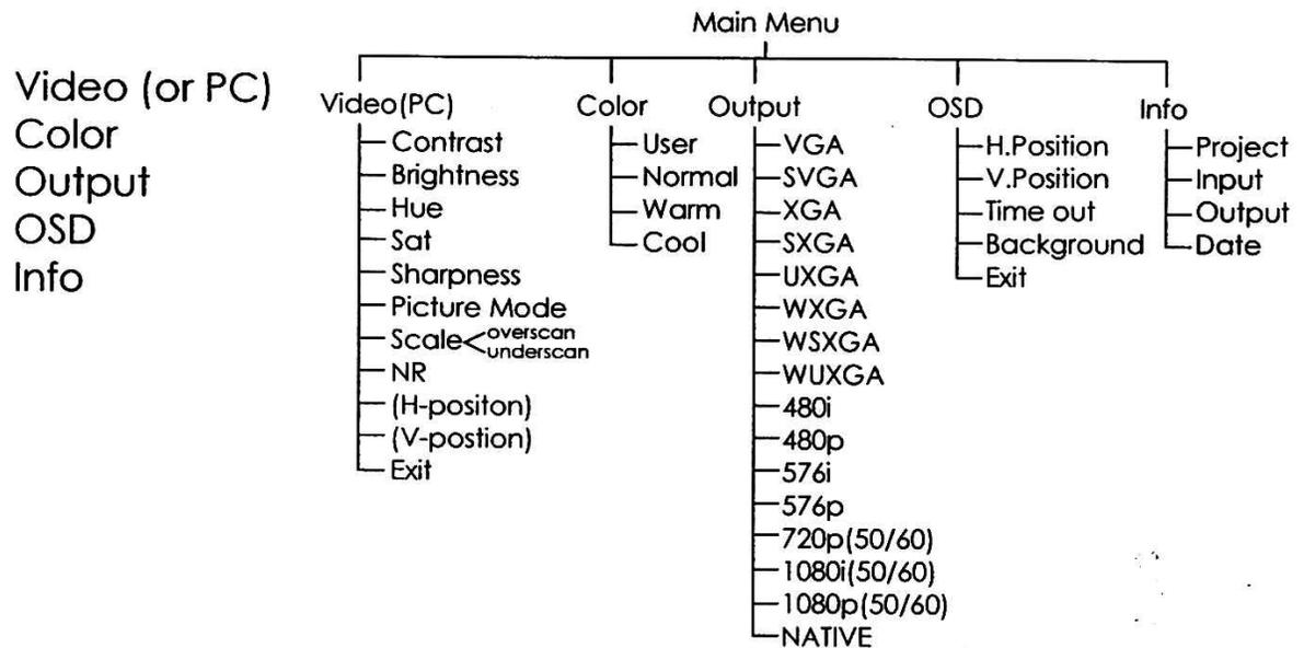
Use +, - button to move highlight bar to your desired parameter, then press MENU/ENTER to enter into sub-menu of your selected parameter.
