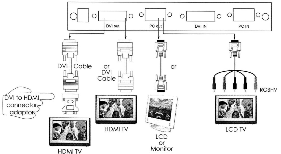
The DVI Digital scaler with ultra high bandwidth can output a variety of PC, SD and HD resolutions in both digital and analog format simultaneously.
