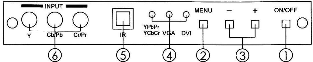
**1. Power:** Press the button to turn ON or turn OFF (standby) the power of the unit.
