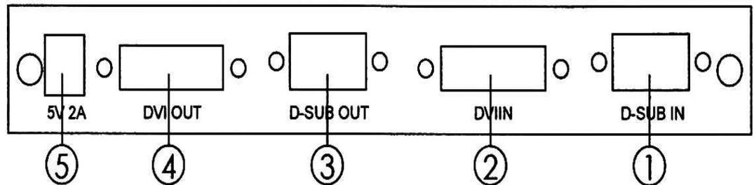
1. **PC input:** Connects this PC input connector to the VGA output of your PC. The acceptable PC resolutions range from VGA-WUXGA.
