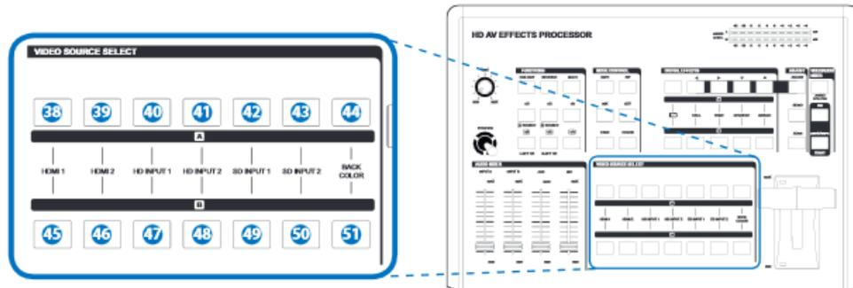
**38/45 :** Used to select Source1,HDMI1. Press both keys together to allow input port HDCP support
