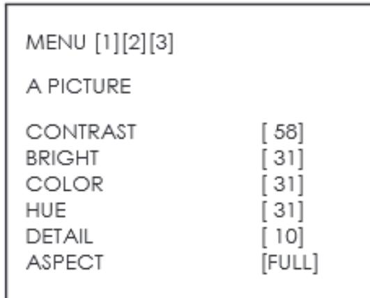
Above values are not save to EEPROM. When the device is turn off the system will change the value back to previous value. Press 28 ADJUST to exit the OSD adjust screen and the system will automatically save to the system.
