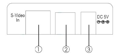
① S-Video input: This slot is where you connect the input source, such as a digital camcorder or a PDA with an S-Video cable in order to send an input signal.
