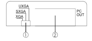
(1) XGA/SXGA/UXGA switch: This dip switch allows you to set the output timing to XGA, SXGA or UXGA. Simply push the dip switch to left, middle or right and the output image will display your desired timing.
