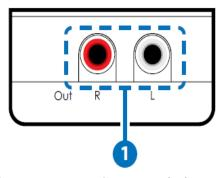
1. R/L Out: Analog stereo output. Connect to the input of your audio device or display.
