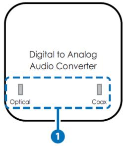
**1. Coaxial/Optical Input Status LED**: The LED light will illuminate according to which input is currently selected.
