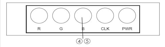
4 Connect BNC-F connectors to both sides of the 5 cables.
