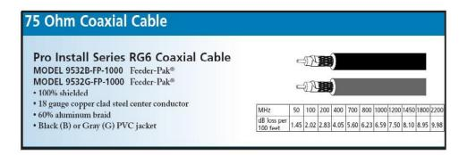
RG6 Type 75 $\Omega$  coaxial cable (for cable TV) x 5 1080P/8bit  $\rightarrow$ 100M 1080P/12Bit $\rightarrow$ 75M
