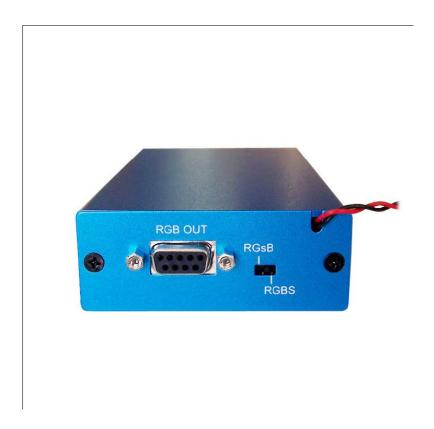
1. **RGBs/RGsB Switch-** This button is used to select between RGBs or RGsB (Sync On Green).
