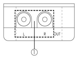
**1. L/R OUT:** These jacks are where you connect an output stereo cable to an amplifier, speaker or TV so you can output audio.
