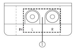
**1. L/R IN:** These jacks are to connect with input sources such as DVD/Blu-Ray players using stereo cables in order to receive an audio signal.
