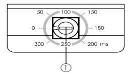
**1. Lip SYNC switch:** This switch has eight settings that allow users to set the audio output delay from  $0\sim300$  milliseconds in order to have perfectly synced audio and video.
