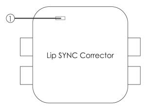
**1. Power LED:** The blue LED will illuminate when the device is connected with power and detected the signal.
