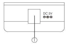
**1. DC 5V:** This slot is where you plug the 5V DC power supply into the unit and connect the adapter to an AC outlet.
