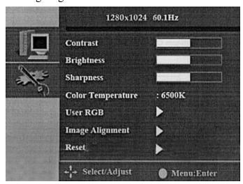
**Please Note:** Due to the advanced nature of this panel. Adjustments to clock, phase and image positioning are saved only for the signal timing you are currently using. Meaning if your input is CGA 640 x 215 @60Hz, and you adjust the clock setting. This will only affect this timing.
