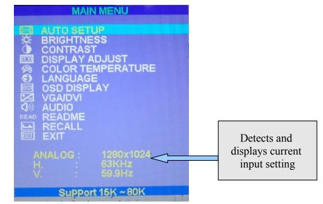
**Please Note:** Due to the advanced nature of this panel. Adjustments to clock, phase and image positioning are saved only for the signal timing you are currently using. Meaning if your input is CGA 640 x 215 @60Hz, and you adjust the clock setting. This will only affect this timing.
