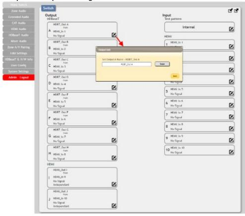
All inputs and outputs can be renamed as required. To rename the HDBaseT output ports and HDMI input ports please click the "edit" icon ( ). Click the "Save" button to confirm the change.
