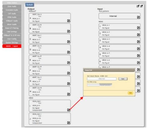
The two HDMI outputs (port I & port J) allow support for the maximum HDMI timing up to 18Gbps (4096×2160@60Hz) and can be used for normal source routing (listed as "Independent" within the WebGUI) and mirroring (listed as "Mirror" within the WebGUI) for local monitoring purposes or zone monitoring (e.g. The HDBaseT output connects to a TV in a remote zone the local HDMI connection goes into an AVR ).
