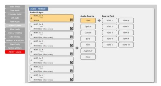
Click the buttons from left to right to choose each output's source. Once the new source has been selected, the change will happen immediately. Audio source options include HDMI, Optical, Coaxial, Line, OAR, Audio CAT and Mixer.
