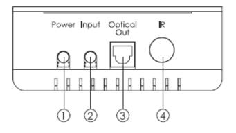
Power: Press this button to turn on the device or to set it to standby mode. The blue LED on the top panel will illuminate when the device is turn on.
