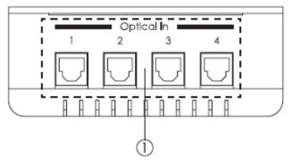
**1 Optical In:** These slots are to connect with input source equipments such as DVD/Blue-Ray player for audio input signal sending.
