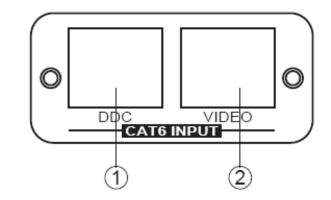
**1. Video input:** Connect the video input to the video output of the transmitter unit using CAT-6 cable.
