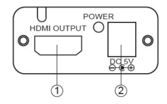
**1. HDMI output:** Connect the HDMI output port to the HDMI or DVI input of your display.
