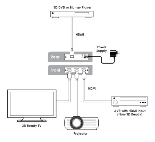
In this example, when the input signal is of 3D format, only HDMI OUT 1 will have picture, while HDMI OUT 2 won't because the projector is non 3D-ready. When the input signal is of 2D format, both HDMI output port 1 and 2 will have picture
